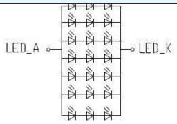
Figure 4.1 LED connection of backlight
